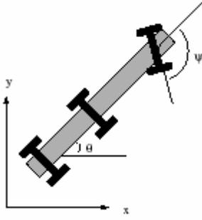
Figure 5: 1 driven and steered wheel, 2 passive wheels
