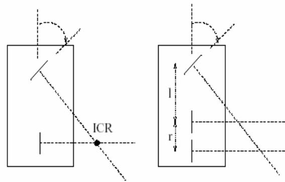
Figure 2: (a) kinematic car; (b) simplified Rocky 7.
