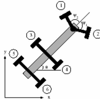
Figure 4: 6 driven wheels, 2 steerable wheels
