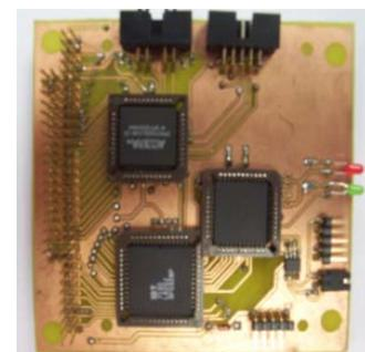
Fig.3 Bus control board
